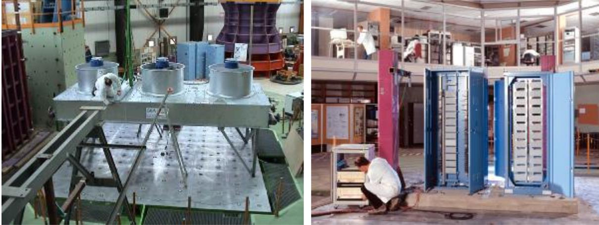
Figure # 3 – Seismic qualification tests on equipment: Cooling system – Electric cabinets
