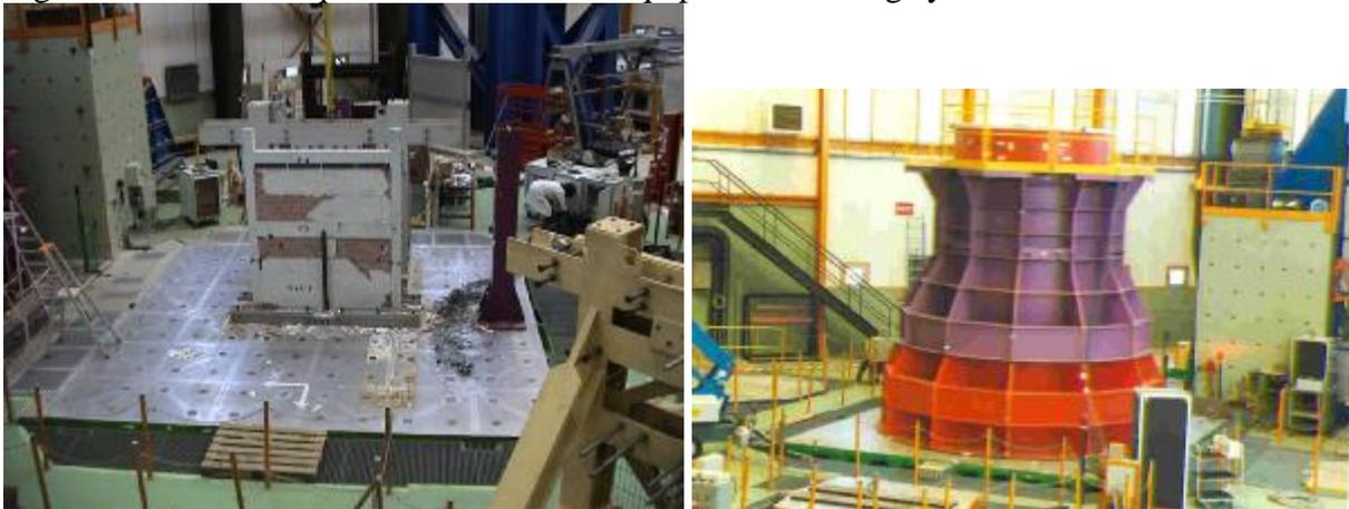
Figure # 4 – seismic tests - concrete frame with masonry – fast breeder reactor core scale 1.
